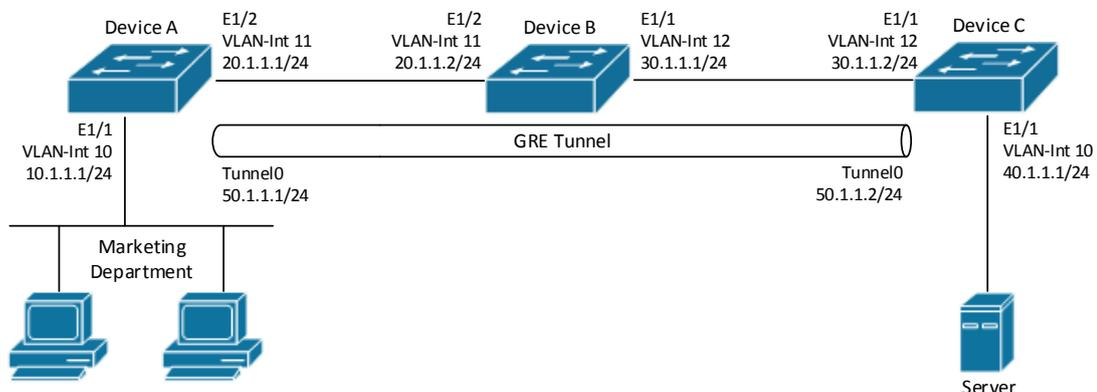
Figure 65.1: ERSPAN application diagram
