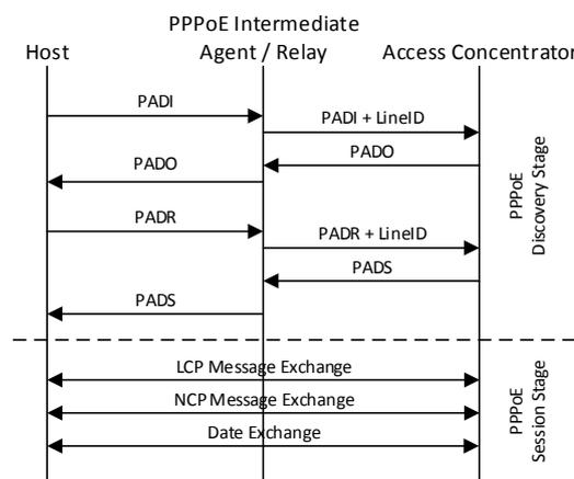
Figure 55.1: PPPoE IA protocol exchange process
