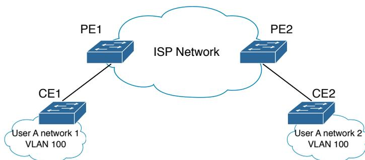
Figure 16.1: BPDU Tunnel application
