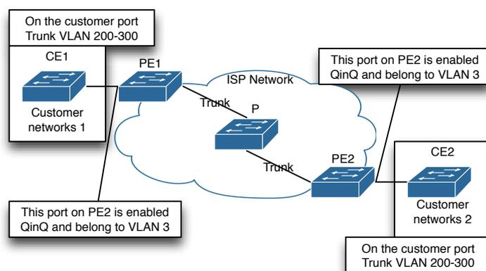
Figure 19.1: Dot1q-tunnel based Internetworking mode
