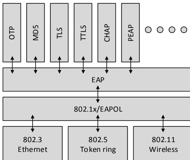
Figure 46.8: the Protocol Stack of EAP Authentication Method
