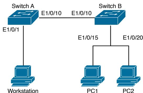
Figure 44.1: Function configuration of the Multicast VLAN
