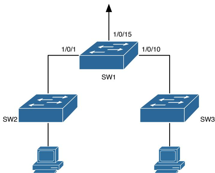
Figure 6.1: Typical example of port isolation function
