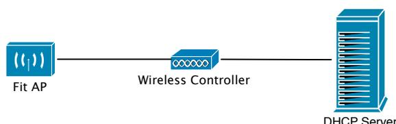
Figure 39.1: Typical DHCP option 60 and option 43 topology
