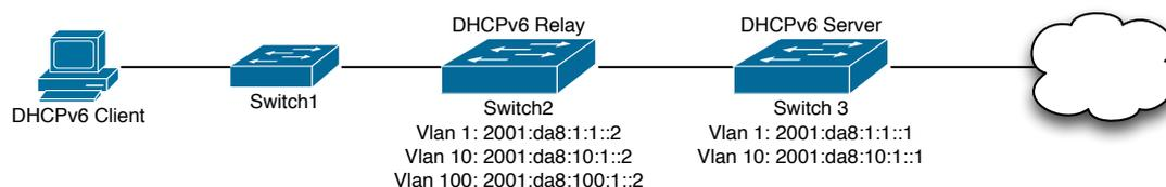
Figure 40.2: DHCPv6 relay option schematic
