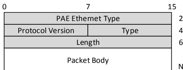
Figure 46.3: the Format of EAPOL Data Packet
