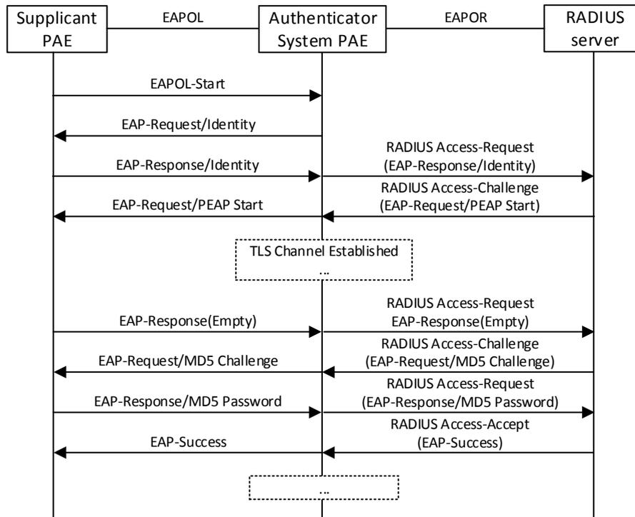
Figure 46.11: the Authentication Flow of 802.1x PEAP
