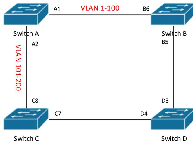
Figure 60.2: VLAN load balance
