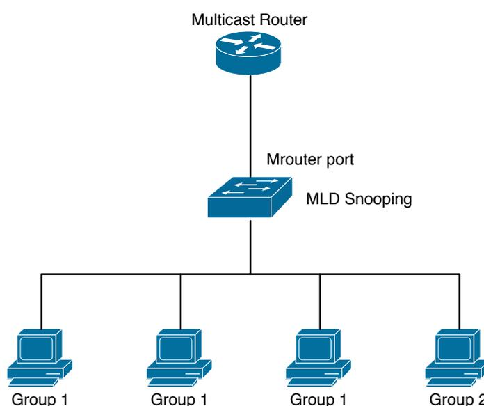
Figure 43.1: Open the switch MLD Snooping Function figure
