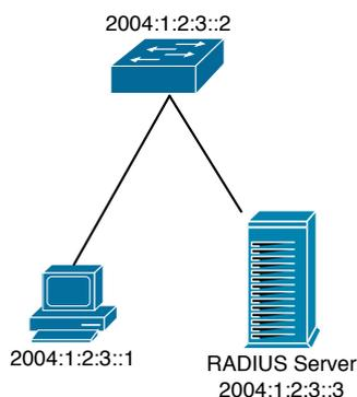
Figure 51.3: The Topology of IPv6 Radius configuration
