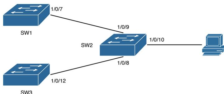
Figure 5.1: Port Configuration Example
