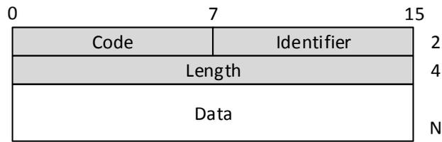
Figure 46.4: the Format of EAP Data Packets
