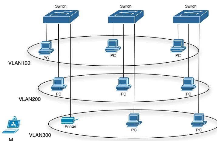
Figure 23.1: Typical topology application of dynamic VLAN
