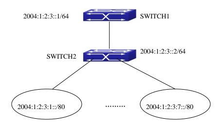
Figure 12-10 IPv6 Black Hole Routing Configuration Example
