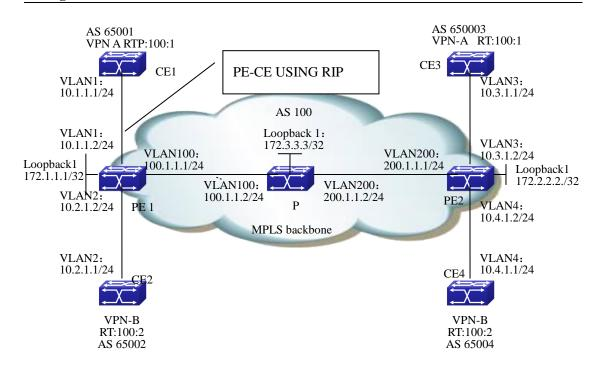
Figure 10-18 Create BGP MPLS VPN between PE-CE via RIP
