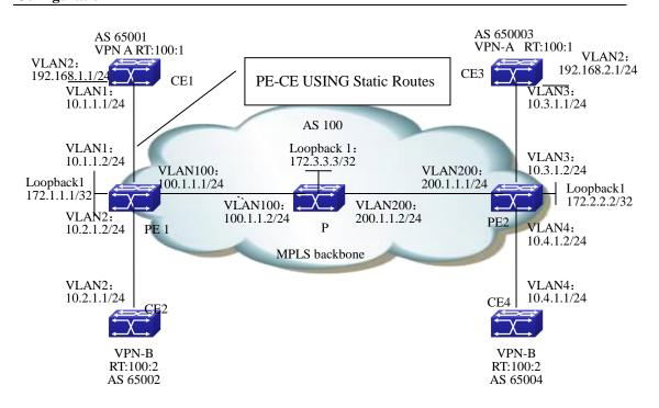
Figure 10-19 Create BGP MPLS VPN between PE-CE via Static Routes
