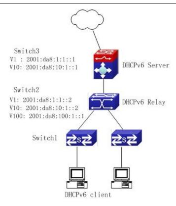
Figure 12-5 DHCPv6 relay option schematic
