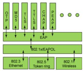
Figure 6-8 the Protocol Stack of EAP Authentication Method
