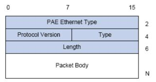
Figure 6-3 the Format of EAPOL Data Packet
