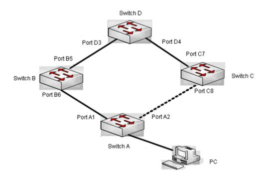
Figure 7-15 the using scene of ULPP
