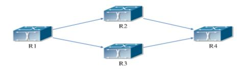
Figure 4-17 the application environment of ECMP
