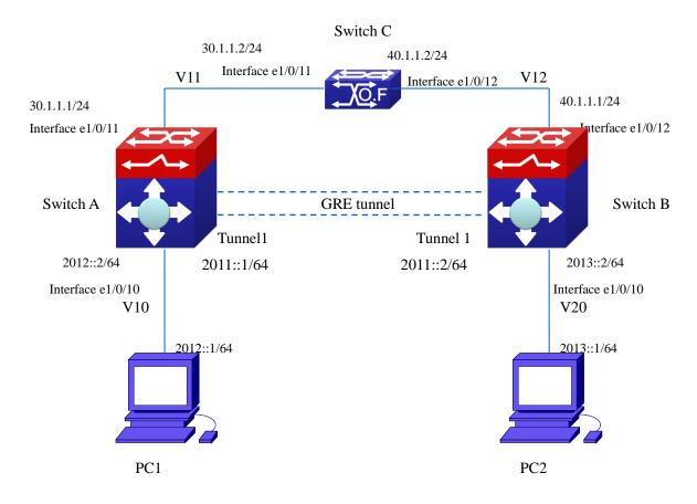
Figure 4-15 the typical network of IPv6 over IPv4 GRE tunnel character
