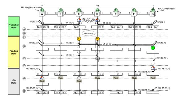
Figure 7-7 Revertive switch fault restoration of single link
