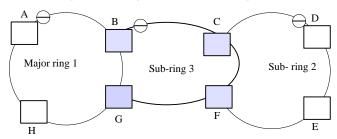
Figure 7-10 the interconnection ring topology without virtual channel
