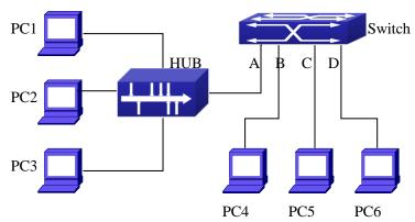
Figure 3-8 ARP GUARD schematic diagram
