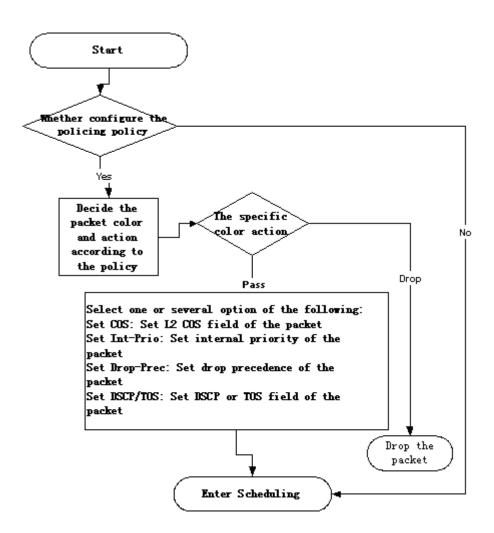
Figure 6-37 Policing and Remarking process
