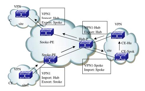
Figure 10-13 Hub&Spoke Networking Resolution
