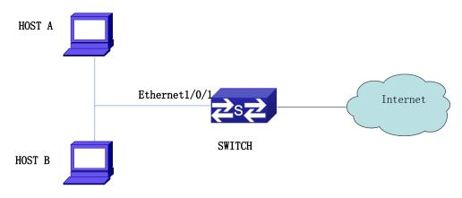
Figure 2-18 Typical topology chart for port security
