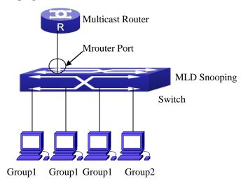
Figure 12-16 Open the switch MLD Snooping Function figure
