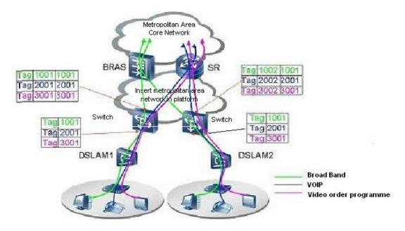
Figure 6-42 Flexible QinQ application topology
