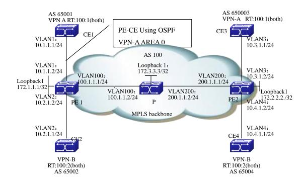
Figure 10-17 Create BGP MPLS VPN between PE-CE via OSPF
