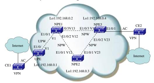
Figure 10-30 H\_VPLS network in LSP access mode
