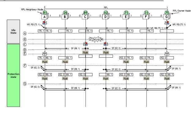
Figure 7-6 single-link fault
