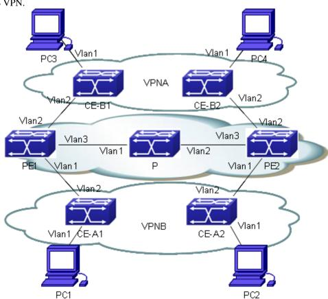
Figure 10-8 MPLS VPN Typical Instance
