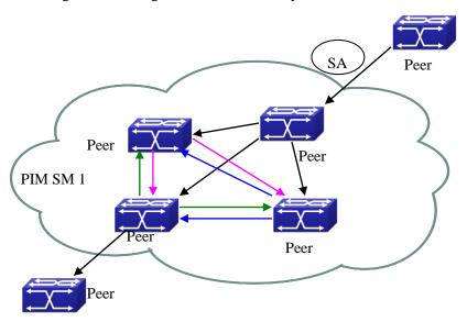
Figure 5-5 Flooding of SA messages
