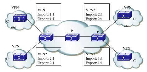
Figure 10-12 Basic VPN Networking Resolution
