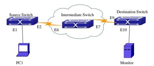
Figure 8-1 RSPAN Application Sample
