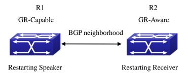
Figure 4-22 Aplication environment for GR
