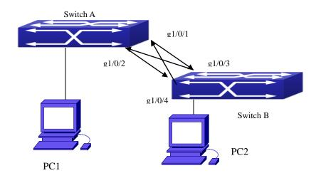
Figure 2-6 Fiber Cross Connection
