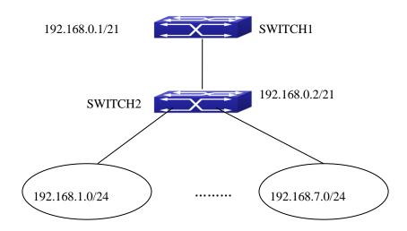
Figure 4-14 IPv4 Black Hole Routing Configuration Example
