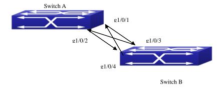
Figure 2-4 Fiber Cross Connection
