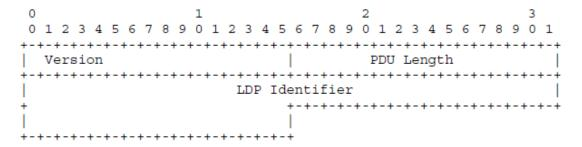
Figure 10-5 The LDP Header Format
