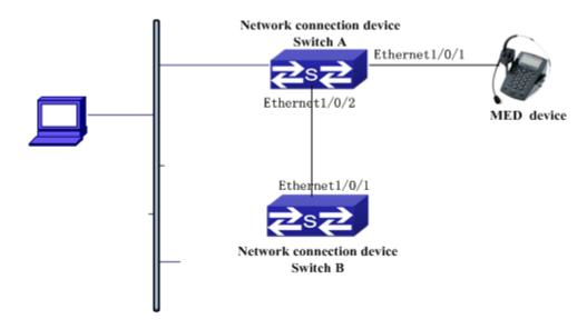
Figure 2-8 Basic LLDP-MED configuration topology
