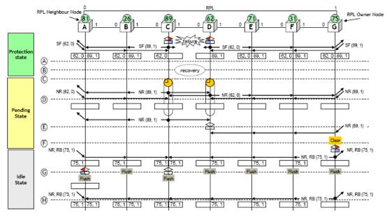
Figure 7-8 Non-revertive switch fault restoration of single link
