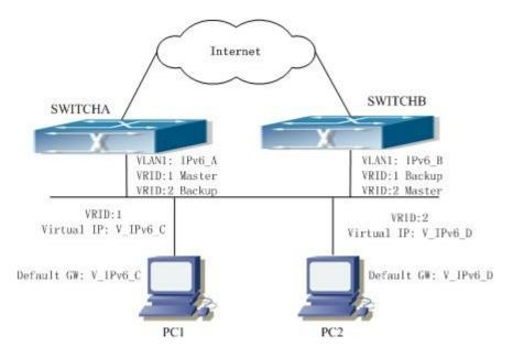
Figure 12-22 VRRPv3 Typical Network Topology
