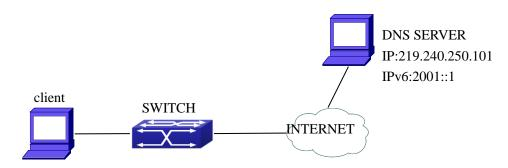
Figure 9-5 DNS SERVER typical environment
