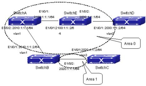
Figure 12-8 Network topology of OSPF autonomous system
