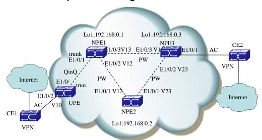
Figure 10-31 H\_VPLS network in QinQ access mode
