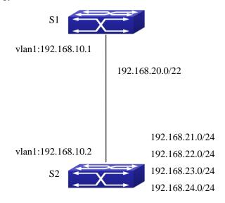
Figure 4-4 Typical application of RIP aggregation
