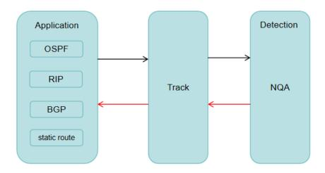
Figure 1-1 Schematic diagram of Track linkage function
