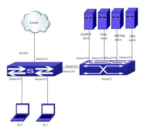
Figure 12-20 IPv6 web portal typical application scene
