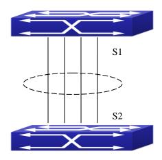
Figure 2-11 Configure Port Channel in ON mode
