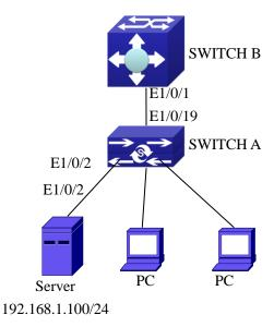
Figure 3-6 ARP scanning prevention typical configuration example
