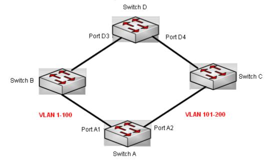
Figure 7-16 VLAN load balance
