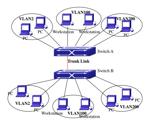
Figure 2-20 Typical VLAN Application Topology
