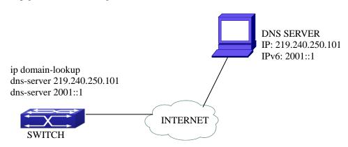
Figure 9-4 DNS CLIENT typical environment
