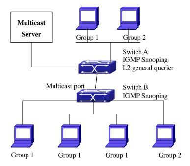
Figure 5-12 The switches as IGMP Queries
