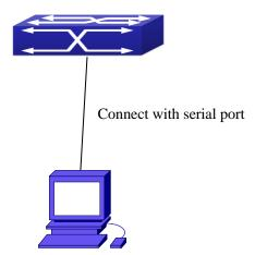
Figure 1-1 Out-of-band Management Configuration Environment
