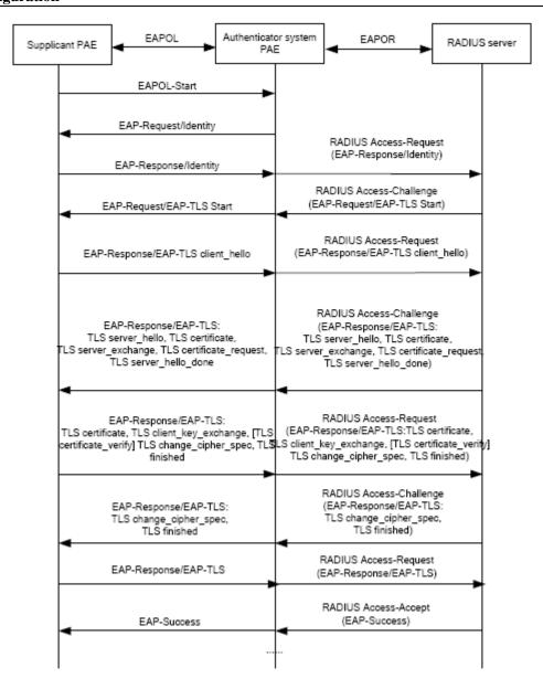
Figure 6-10 the Authentication Flow of 802.1x EAP-TLS
