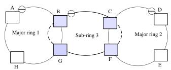
Figure 7-9 the interconnection ring topology with virtual channel
