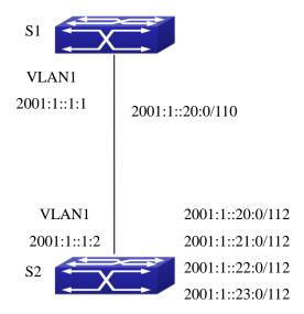
Figure 12-7 Typical application of RIPng aggregation
