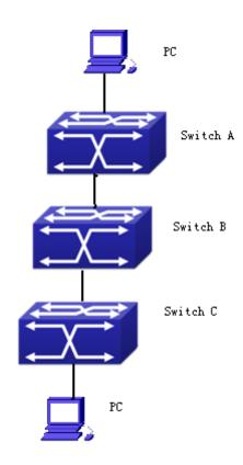
Figure 2-23 Typical GVRP Application Topology
