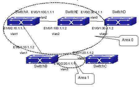
Figure 4-5 Network topology of OSPF autonomous system
