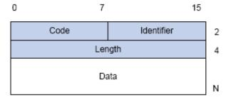
Figure 6-4 the Format of EAP Data Packets
