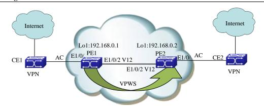
Figure 10-32 VPWS group network diagram
