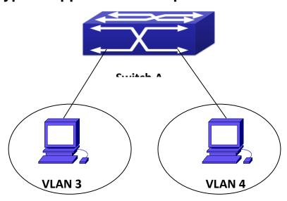
Figure 2-31 typical of super vlan topology
