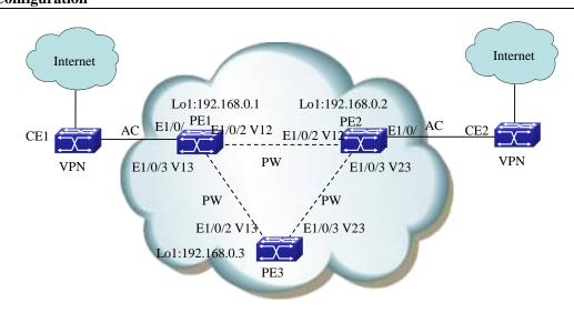
Figure 10-29 full connection VPLS model for PE
