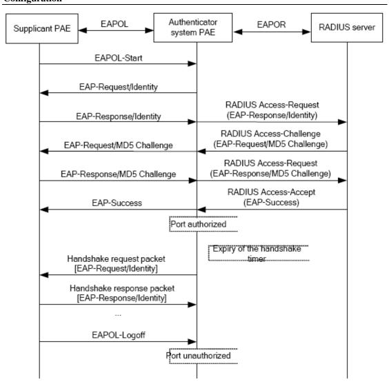
Figure 6-9 the Authentication Flow of 802.1x EAP-MD5
