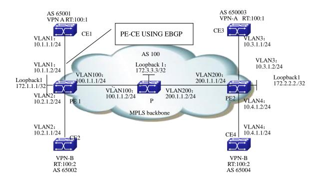
Figure 10-16 Create BGP MPLS VPN between PE-CE via EBGP
