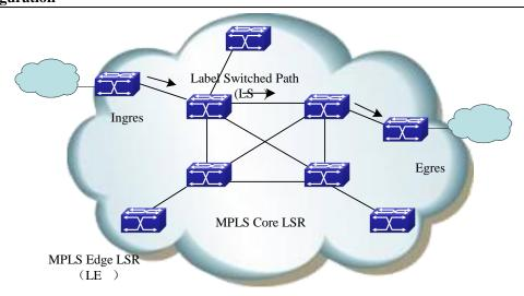
Figure 10-3 The MPLS Network Structure
