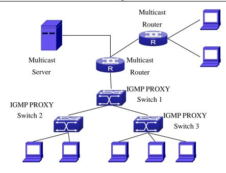
Figure 5-13 IGMP Proxy Topology Diagram
