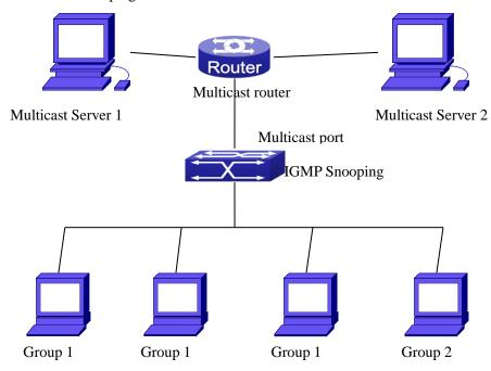
Figure 5-11 Enabling IGMP Snooping function
