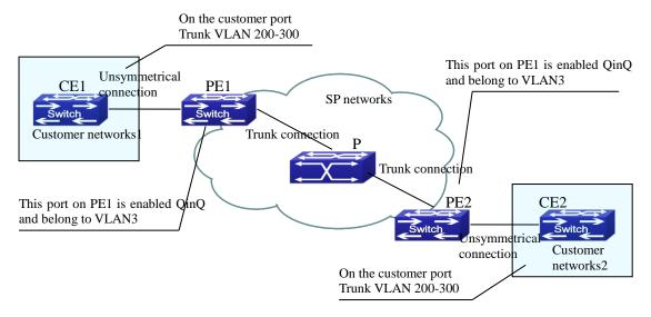
Figure 2-24 Dot1q-tunnel based Internetworking mode
