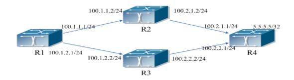
Figure 4-18 the application environment of ECMP
