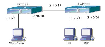
Figure 5-15 Function configuration of the Multicast VLAN
