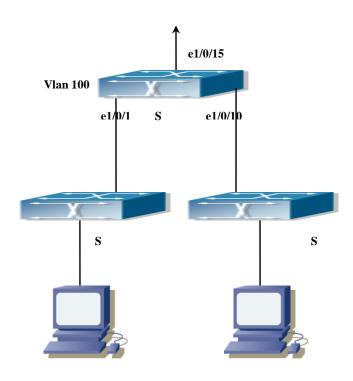
Figure 2-2 Typical example of port isolation function
